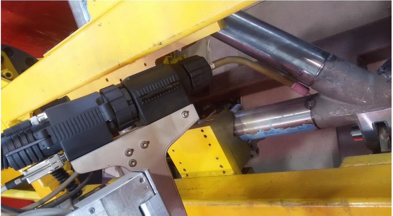
*Special torch LKTZ with Push-Push drive MEP 200: Thanks to its slim shape and the special bending angle, it allows optimum component accessibility*
